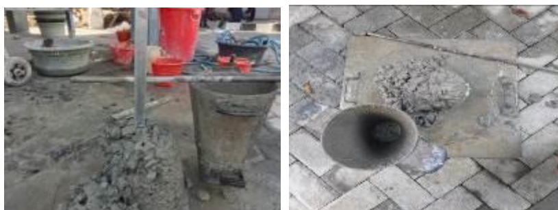
Figure 3: Concrete Slump Test Process
