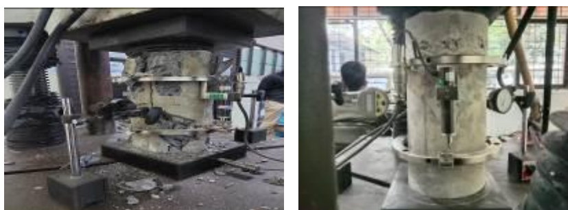
Figure 9: Concrete Elasticity Modulus Testing Process
