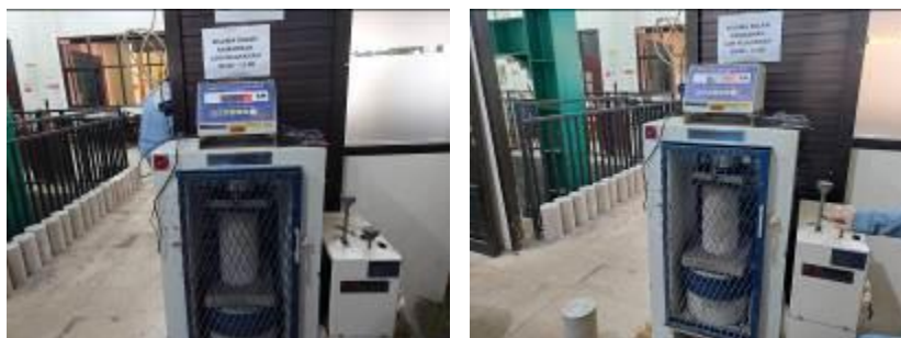
Figure 5: Concrete Compressive Strength Testing Process
