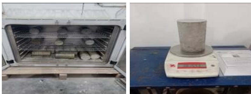
Figure 7: Concrete Porosity Testing Process
