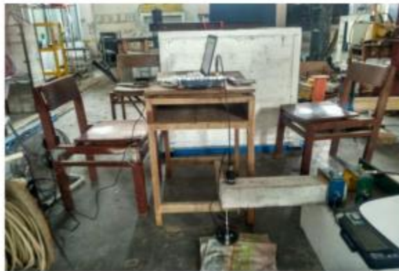
Figure 3. Damping test setup of mortar specimens under free vibration conditions
