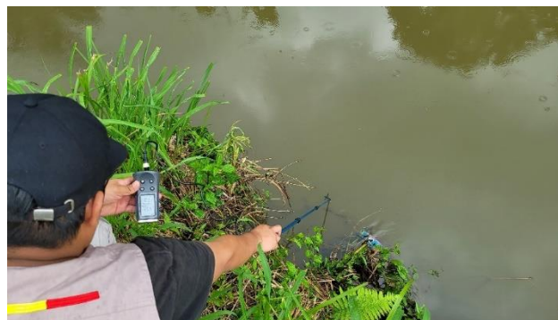
Figure 6. River Water Speed Measurement with Current Meter
