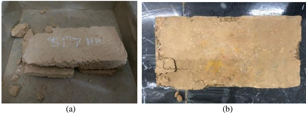
Figure 5. Normal brick (a), 8% Bacteria variation bricks (b)
