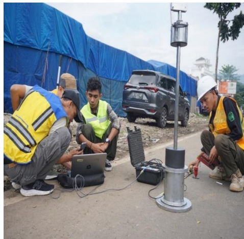
Figure 2. Field Testing of LWD Tools
