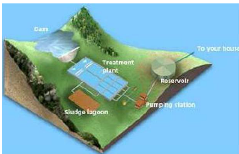
Figure 1. Intake – IPA – Reservoir Scheme
