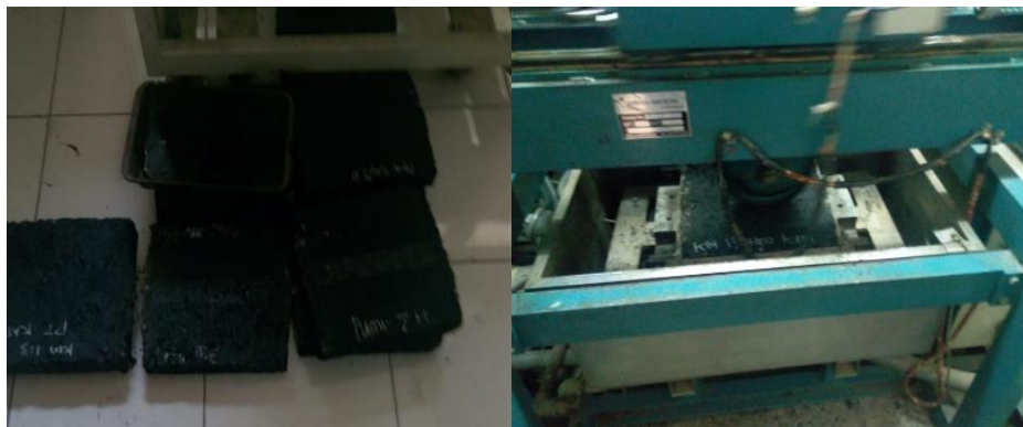
Figure 1. Test Objects and Wheel Tracking Test Equipment
