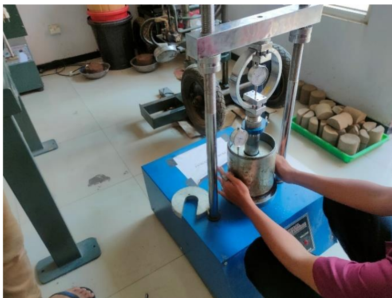
Figure 4. CBR ( California Bearing Ratio ) Test Process
