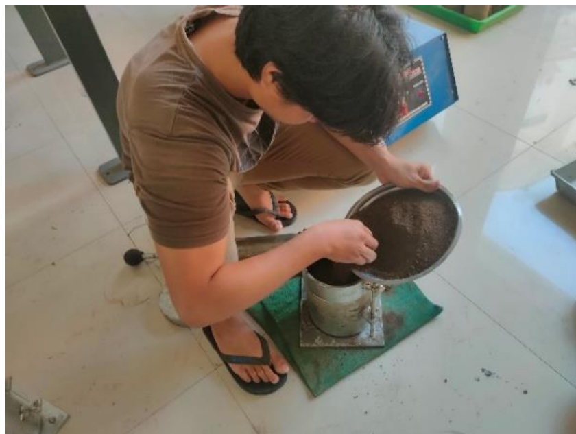
Figure 2. Inserting a Subgrade Soil Sample into a CBR Test Mold
