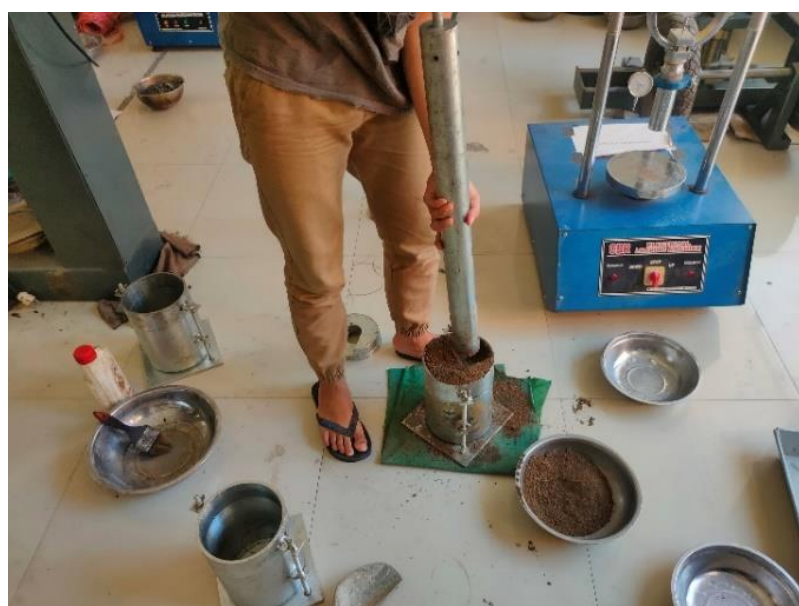
Figure 3. Subgrade Soil Compaction Process
