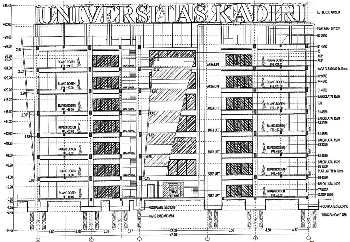
Figure 1. Sectional image of the building during planning
