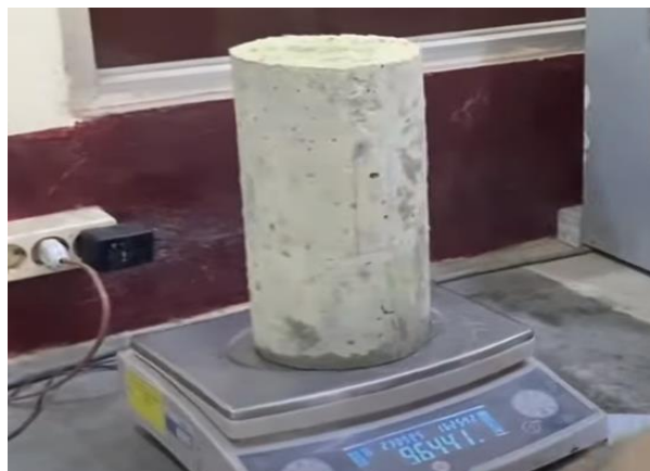
Figure. 4. Weight Testing Dry Density Foamed mortar
