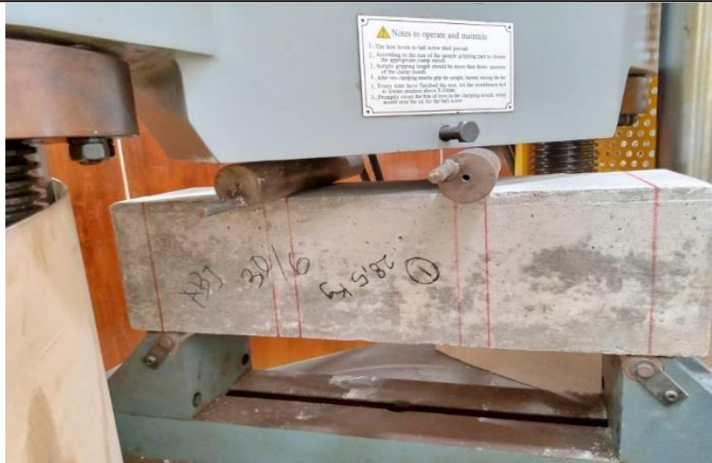
Figure 5. Flexural strength testing
