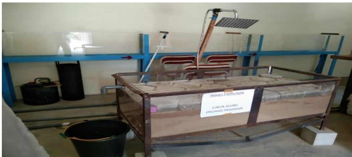
Figure 1 : Infiltration Testing Tank
