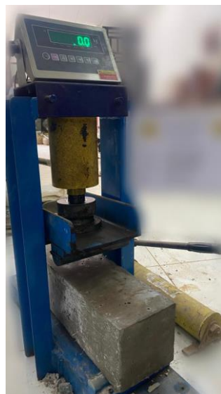
Figure 2 Two Point Bending Test Equipment Loading
