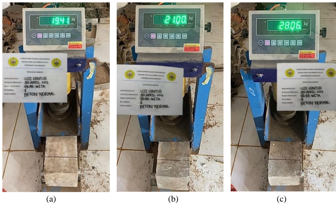
Figure 5: 14 Day Flexural Strength Test Reading (kN) (a), (b), (c) Test Objects
