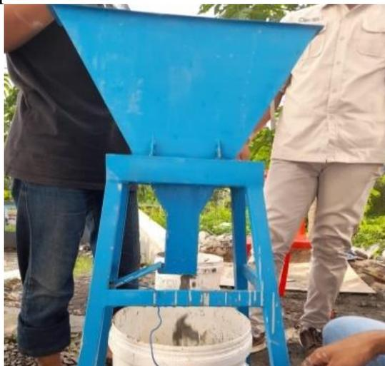
Gambar 2. Uji V-Funnel Tester
