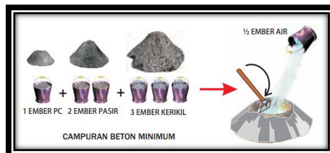
Gambar 9. Campuran Beton Minimum
