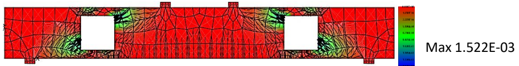
Figure 5: Crack pattern of LPB2 beam
