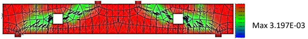
Figure 4: Crack pattern of LPB1 beam
