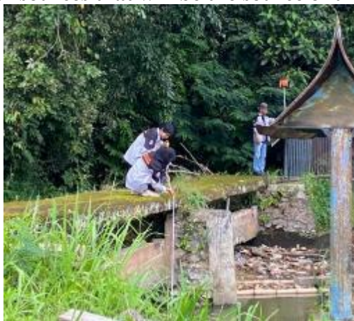
Figure 3: Measurement of Hydraulic Head
